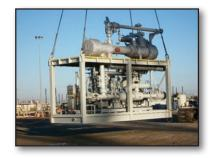
Process skid consisting of receiver barrel, piping and heat exchanger. Design pressure was 10,000#. Skid size was  $8'W \times 21'L \times 18'H @ 33$  tons.
