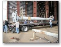
Launcher/Receiver barrels being loaded out in the fabrication shop area. Barrels were  $32'' \times 16'' \times 33'$  long @ 16 tons (left) and  $24'' \times 16'' \times 33'$  long @10 tons (right). Both barrels were 3,700# design pressure.
